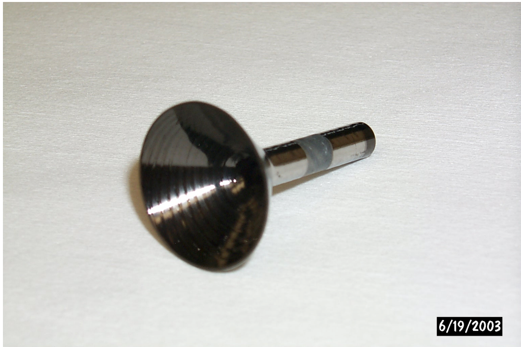
Figure 16. Quad Spiral Channel Electron Multiplier
