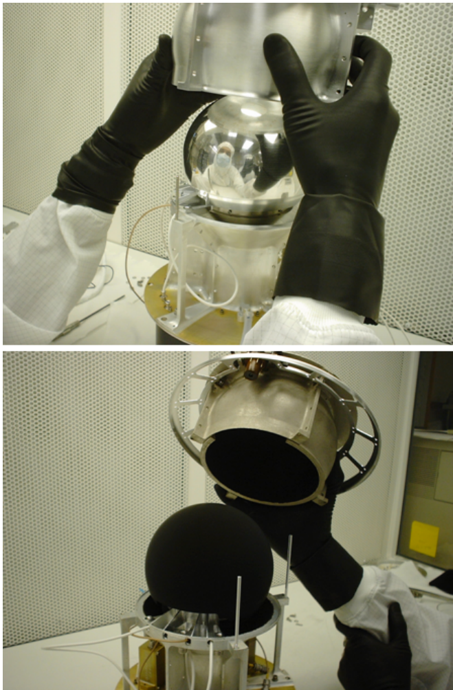
Figure 14. Cantilevered Inner-ESA dome with (bottom panel) and without (top panel) blackening.
