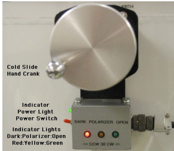
Fig. 13 Cold Dark Slide hand crank and indicator
