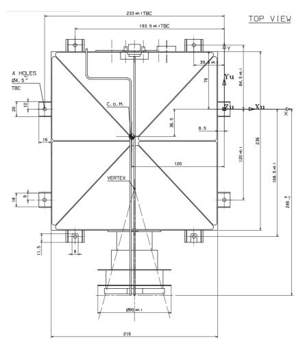
Figure 4: MIDAS with URF system shown at the reference hole
