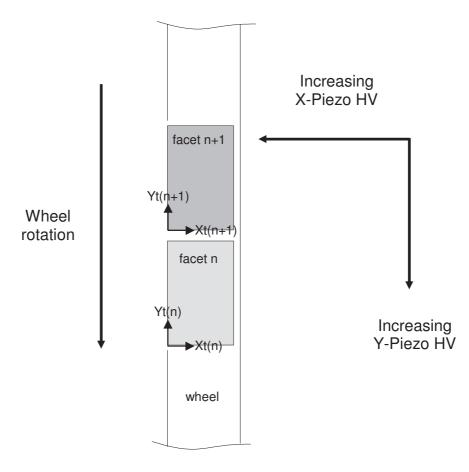
Figure 6: TRF co-ordinates on a target area (facet)
