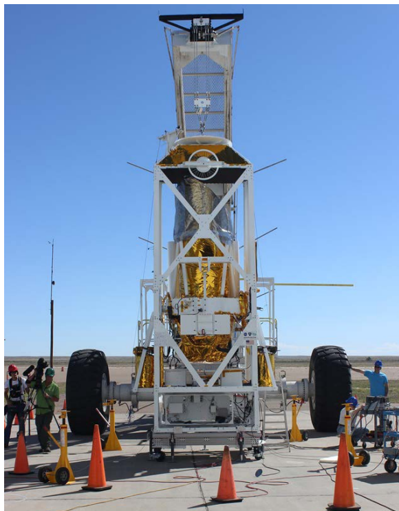
Figure 17 Gondola suspended outdoors from the launch vehicle during the compatibility test.
