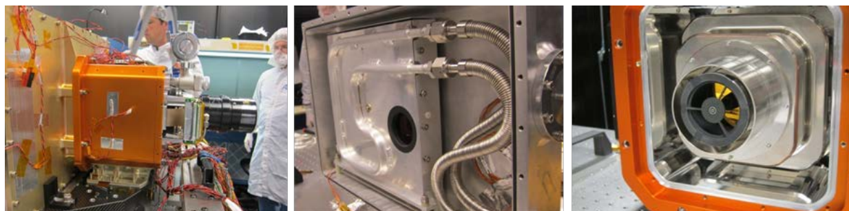
Figure 4. (left panel) the IR camera (orange) and cryocooler (black); (center) the cryogenic filter wheel housing with LN 2 cooling loop; (right) the mini-RC telescope within the IR camera.
