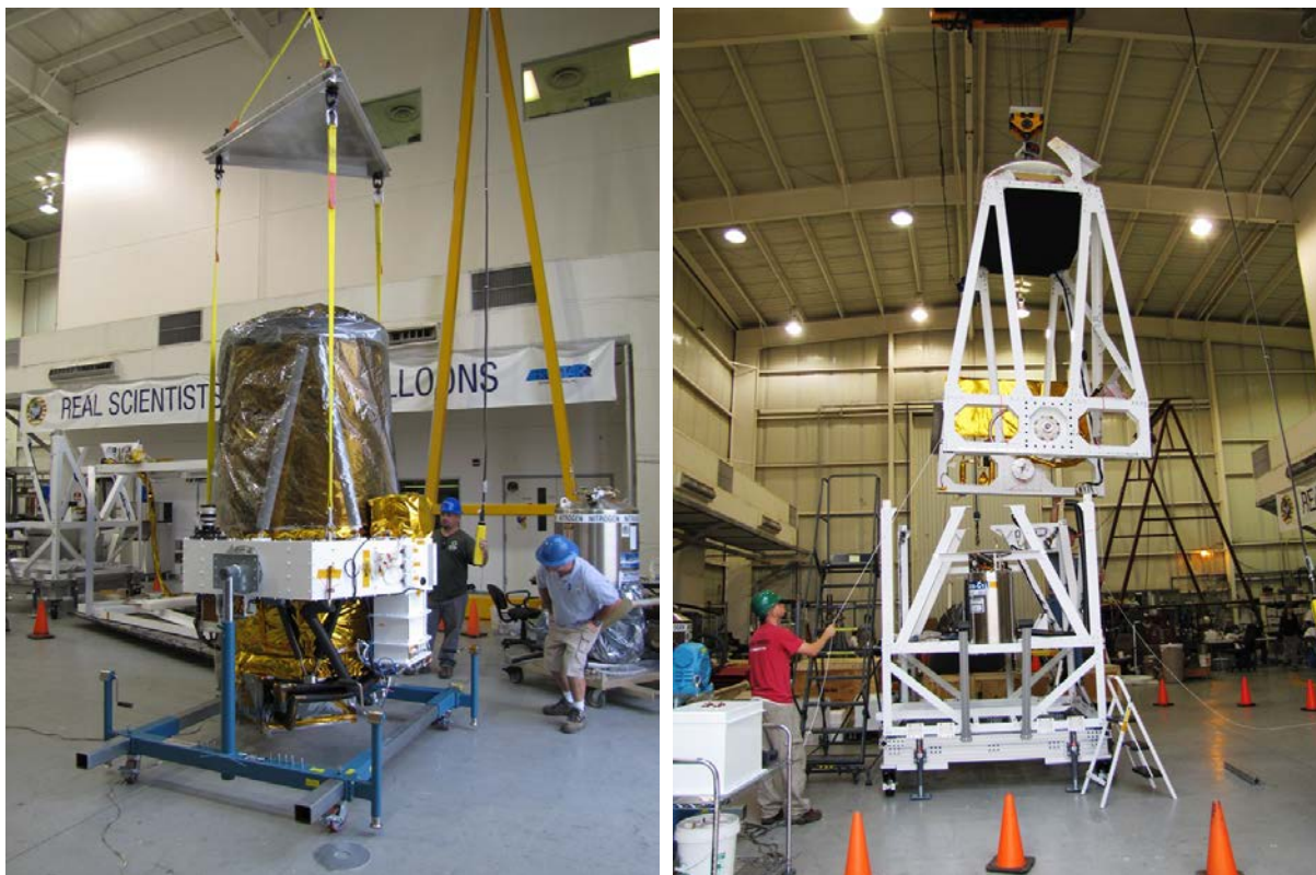
Figure 13 (Left) Installation of the telescope/instruments assembly on the Flotron. (Right) Gondola upper structure is installed on top of gondola baseplate.
