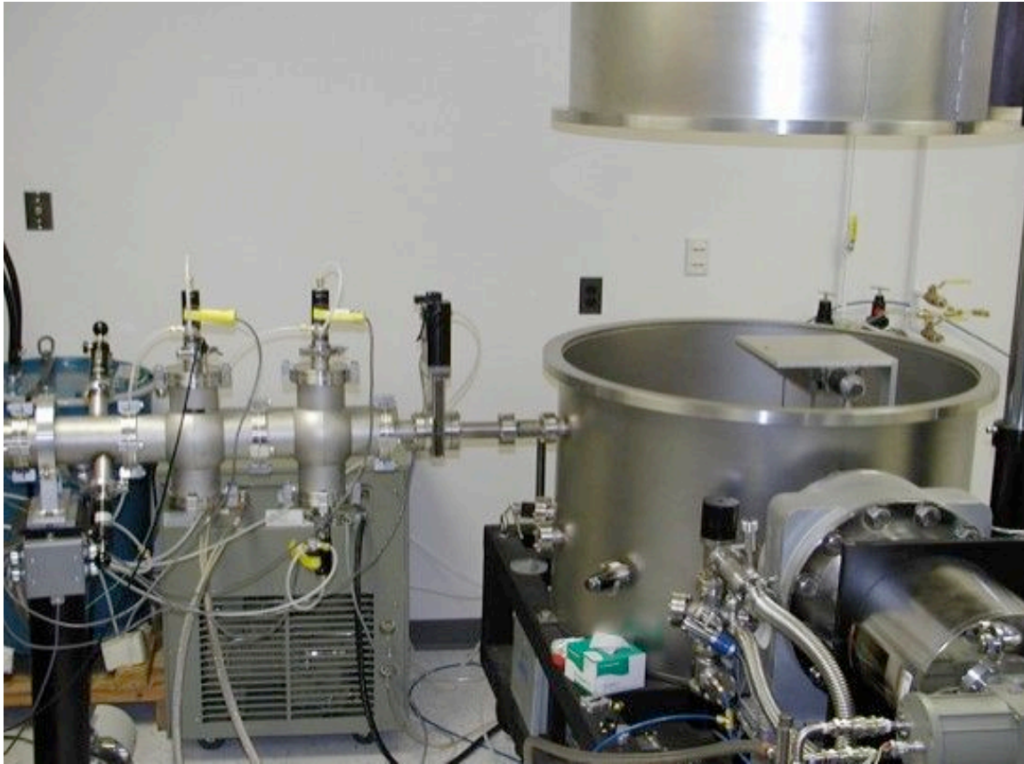
Fig. 21. The vacuum chamber used in calibrating the PEPSSI unit. The beam line enters the chamber horizontally from left to right in the picture.
