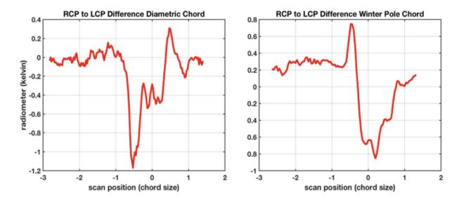
Note: Left side is the Diametric Scan, and right side is the Winter Pole scan. Negative values result from RCP temperatures lower than LCP temperatures..
