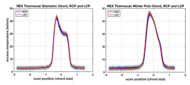
Note: The grey bar indicates the uncertainty in the temperatures due to systematic error in determination of the X-band receiver noise temperature and the REX unit to Kelvin conversion constant.
