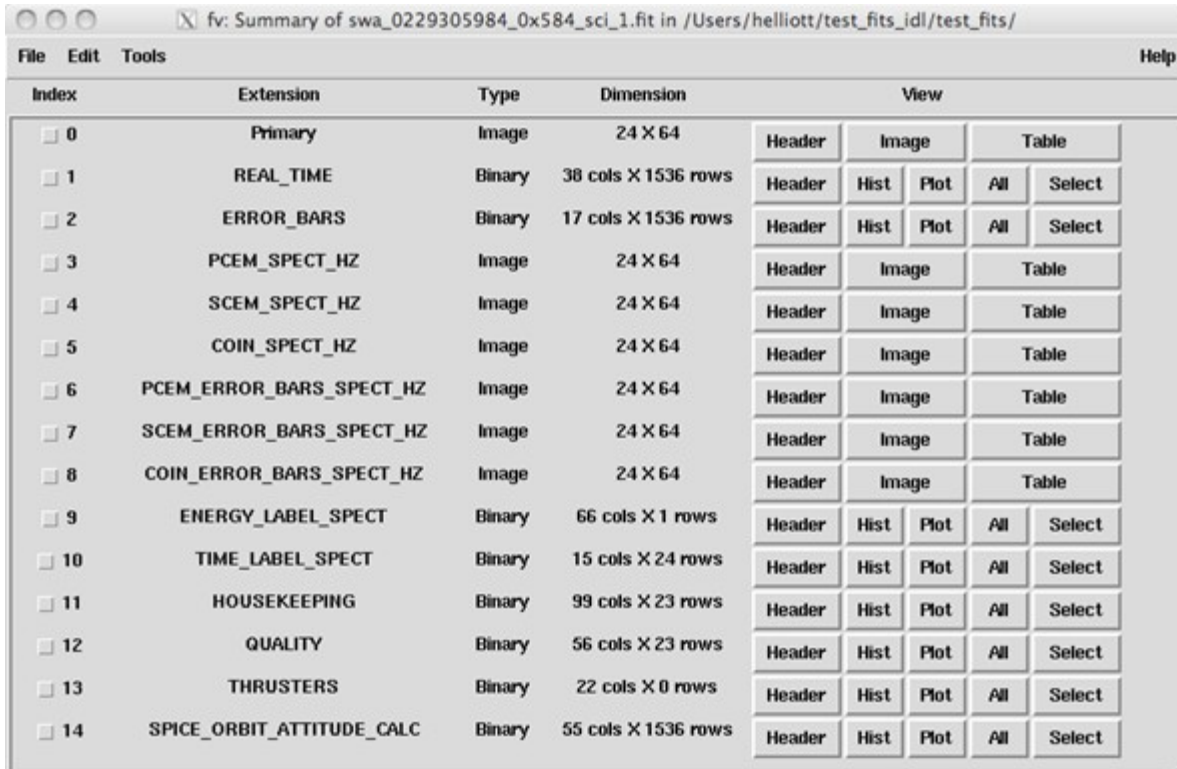
Figure 14-7: Picture of what the real-time calibrated (level 3) files look like using Fv. The numbers listed under index are the extension numbers. All tables are Binary type and all images are image type.
