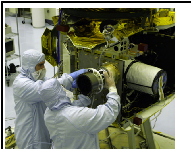
Figure 14-3: Picture of SWAP being mounted to the spacecraft.
