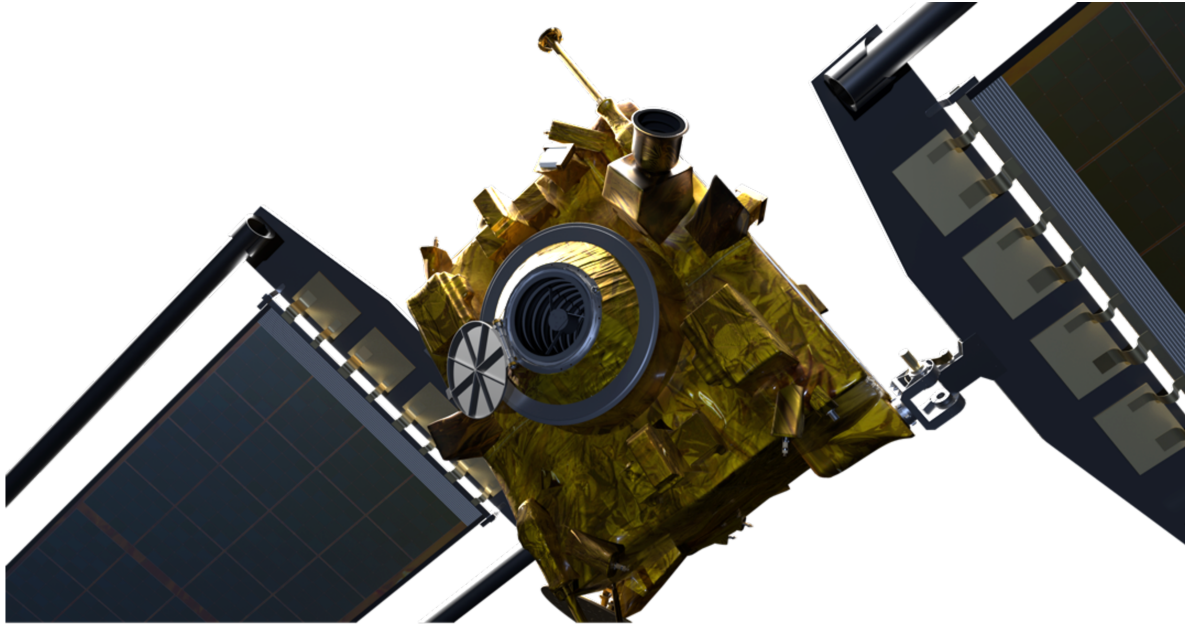
Figure 2. Location of DRACO on the DART spacecraft. The cover is shown in its open position.
