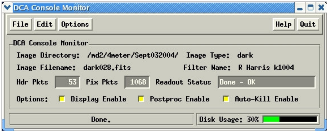
Figure 4.11.1: The main GUI panel for the DCA. Verify that the directory shown is where you want your pictures to go (controlled via the Arcon IRAF window using "cd"). You can watch the packets count up as the picture is read out.
