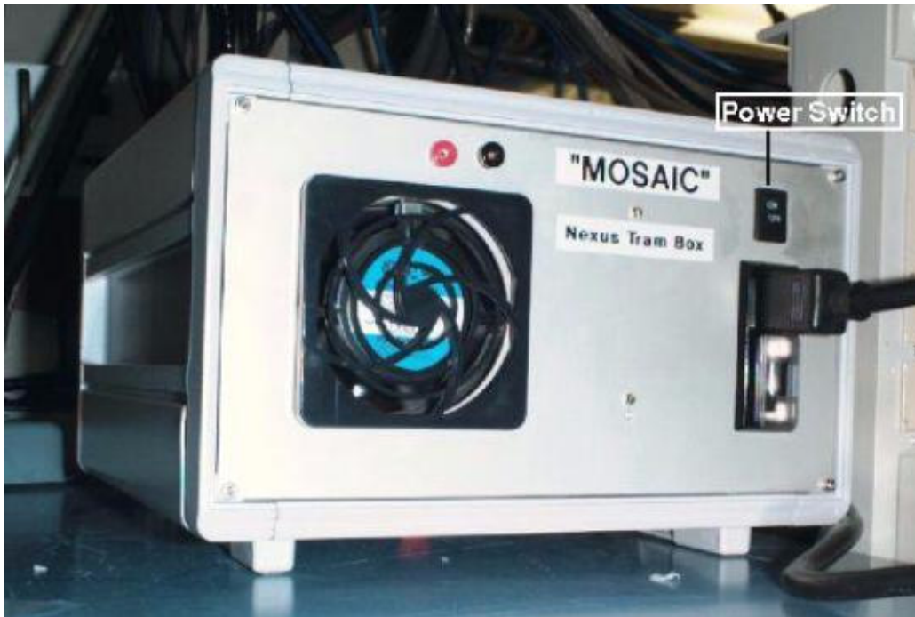
Figure 4.4.1: The Arcon "TRAM" box with Power Switch noted. At the KP4m you should not need to use this switch - see section 10.2.
