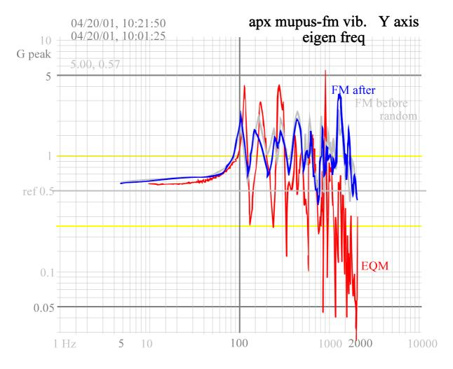
Fig. 7 Response on vibrations in the tests of eigen-frequencies in axis Y
