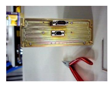
Remove all 6 M2 Screws from the frontplate. Thereby hold the whole stack in your hands to stabilize the loosened stack.
