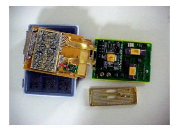
Flap the MPAe power board to the side. Use some supporting box as the cable bundle is too short to place the powerboard at the ground. Loose the 2 M2 screw on the small interface board. Then lift the interface board with the tongs from the lower stacks. Lift only in small steps from all four directions.
