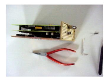
Picture A) shows the assembled board and the used tools (  $\ tong \ with \ flat \ heads \ and \ an \ imbus \ screwdriver \ for \ M2$  )
