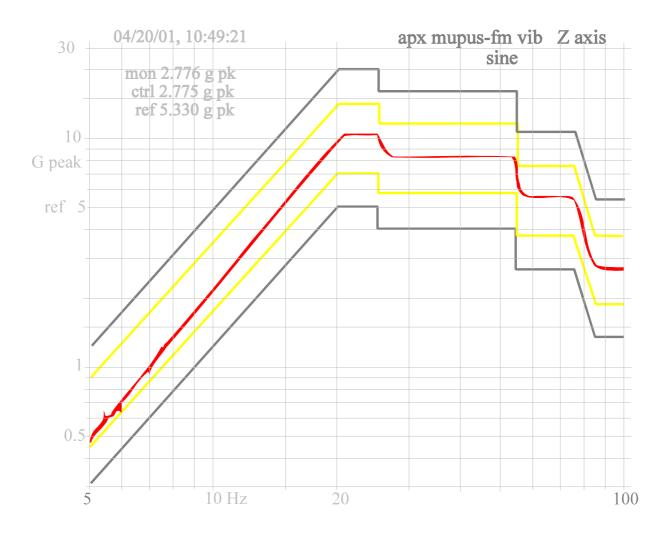
Fig. 11 Response on sine vibrations in axis Z
