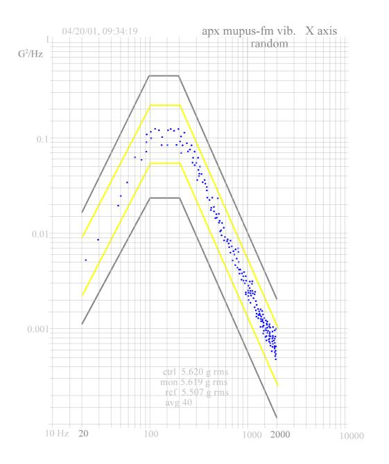
Fig. 6 Response on random vibrations in axis X
