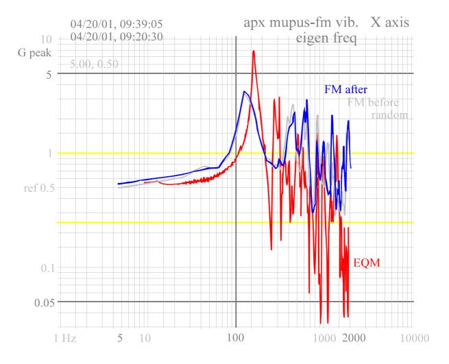
Fig. 4 Response on vibrations in the tests of eigen-frequencies in axis X
