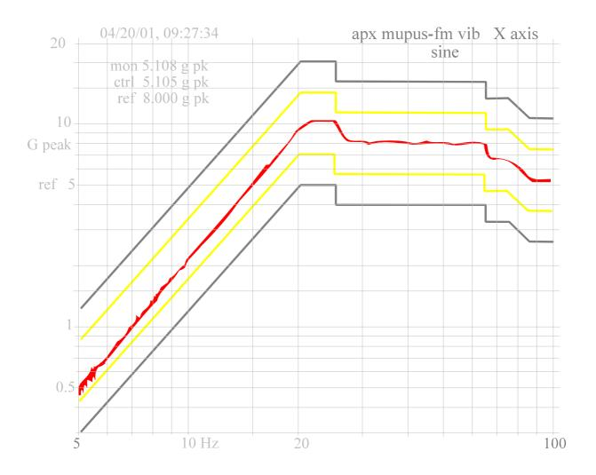
Fig. 5 Response on sine vibrations in axis X
