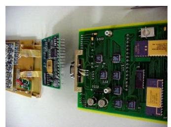
Now loose the 2 M2 screws on the digital board. You can then disconnect the 2 APXS boards with the tongs. First loose the two pin connectors at the front side then disconnect the broad pin connectors at the back side.
