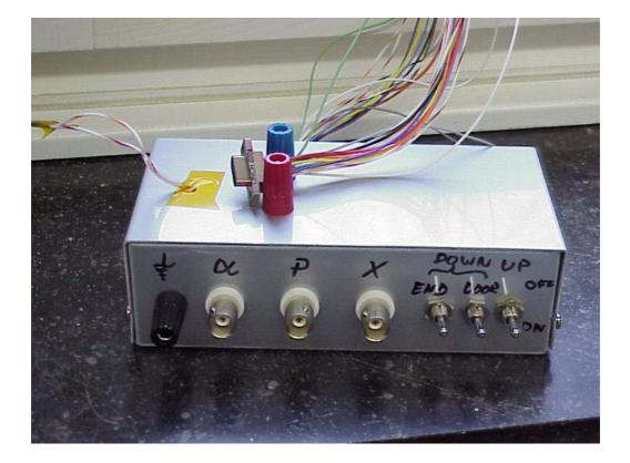
Figure 7: APX Deployment device simulator with connector for J155
