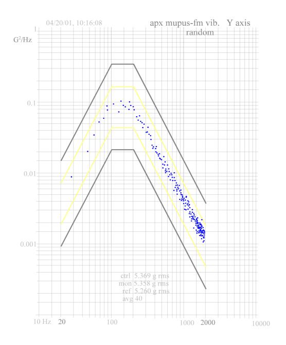
Fig. 9 Response on random vibrations in axis Y
