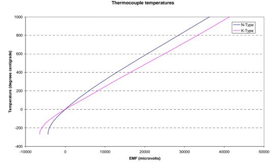
Plot of temperature reading against thermocouple emf for type K and type N thermocouples. Data plotted from Appendix A.
