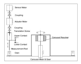
Figure 5 Carousel and Volume Checker Kinematics
