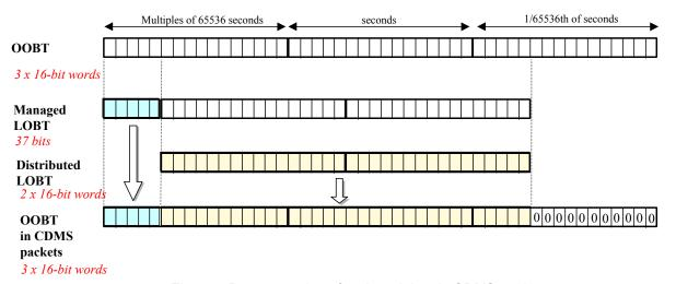
Figure 7 Reconstruction of on board time in CDMS packets
