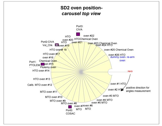
Figure 6 Reference system of carousel
