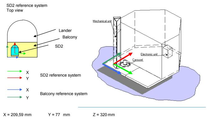
Figure 9: SD2 reference system versus Balcony reference system
