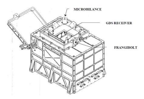
Figure 1 External view of GIADA with cover open
