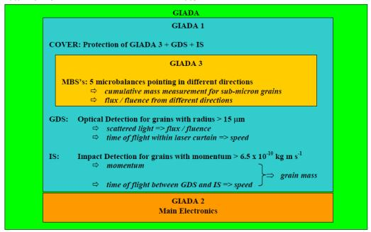
Figure 2 Block diagram of GIADA and performed measurements
