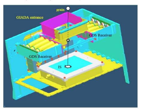
Figure 3 Sketch of the internal configuration of GIADA, where entrance, GDS receiver
