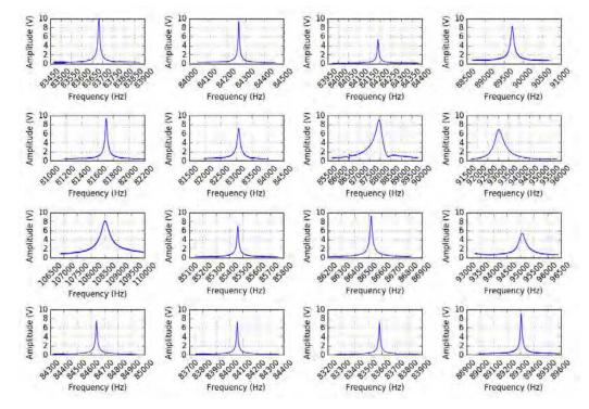
2016-02-10 05:10:00 : Frequency survey of all cantilevers using default parameters:
