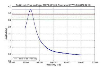
Figure 1: A frequency scan of cantilever 7, used for the majority of scans post -hibernation until the end of 2014. The blue line represents the peak amplitude, the red line the working point (driving amplitude/frequency) of 90% peak and the green line is the set-point of 80%. A re-tune threshold of 85% is given by the dashed line.
