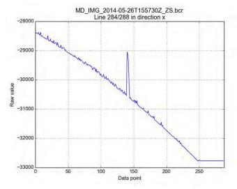
Figure 1. Z piezo extension (y axis in raw instrument values) during scan STP004-3, showing Z piezo reaching maximum extension towards the end of the scan.
