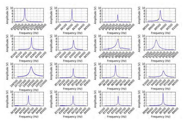
2016-05-25 05:10:00 : Frequency survey of all cantilevers using default parameters
