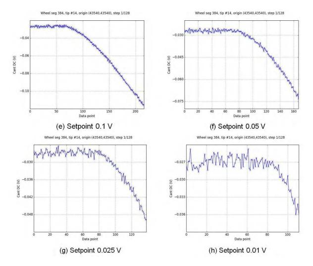
Figure 3: Setpoint variation for a z step size of 4 (a-d) and 8 (e-h) on a solgel target revealing a possible reduction of setpoint down to 0.025 V (c) and (g).
