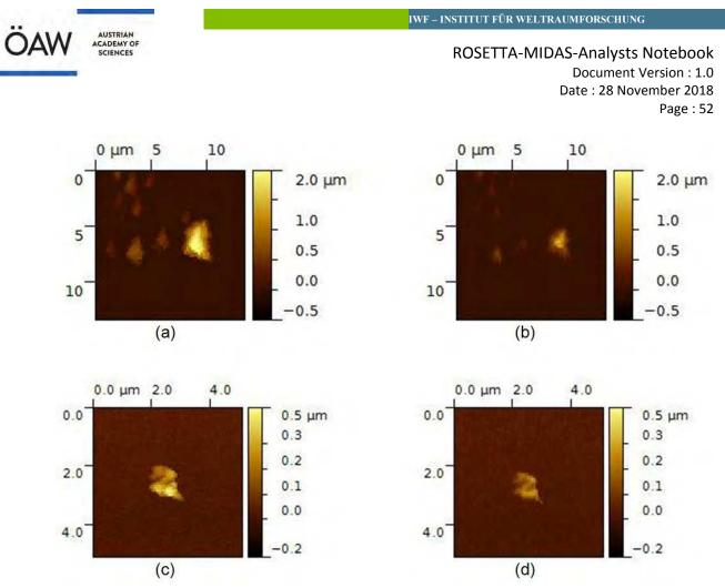
Figure 21: Topography image of a cometary particle with tip 7 (a) and with tip 9 (c). The particle size is in both cases in the order of 2-4  $\mu$ m and the size is from approximately 450 nm to 2  $\mu$ m for the particle in (c) and (a) respectively. (b) and (d) show the deconvoluted image where the tip was taken from figure 3.03. Both show a decreased structure height and other artefacts.
