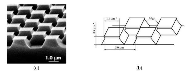
Figure 11: X/Y calibration target. (a) showing an SEM image and (b) revealing the dimensions of this target, which is used for the open loop and hybrid mode comparison.
