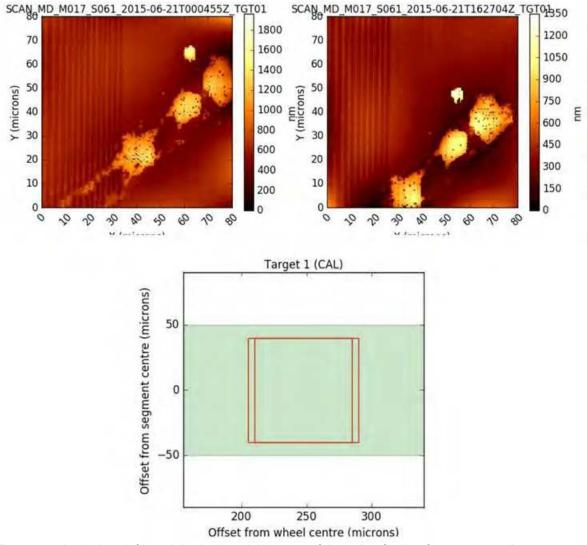
Figure 27: tip 10 (top left) and tip 15 (top right) scan of the edge finding feature, revealing a correct offset in X direction, but showing an offset in Y direction of approximately 15-20  $\mu$ m. The bottom illustration is showing the X corrected positions, but the nominal Y position is still showing the same value, which is clearly not the case when looking at the two scans.
