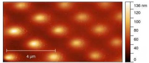
Clearly this is in some way reflective of the tip shape, but the image is very noisy and the height is very small.
