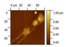
Figure 26: Topography scan of a noticeable structure, which was found at the Z calibration target at the end of the linear grid and used as a marker position to re-calibrate the linear stage.
