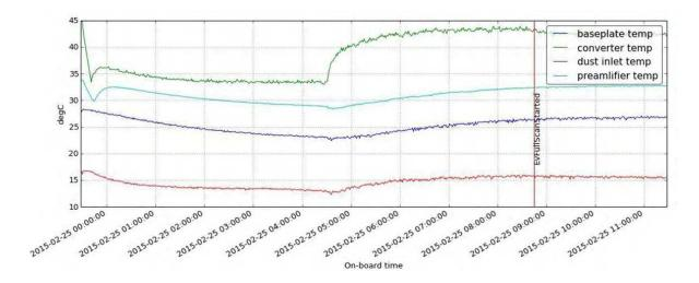
Figure 5: Temperature curves of the four sensors at a reboot at the start of STP 45, showing the decreasing temperature at the left side of the graph at the shut down at 23:30. After the restart at 23:44 only one frequency scan was performed till the end of the OCM at approximately 04:30. For warming the microscope up four approaches were performed till the first scan after the reboot at 09:00, where the temperature gets approximately saturated and allows stable performance.
