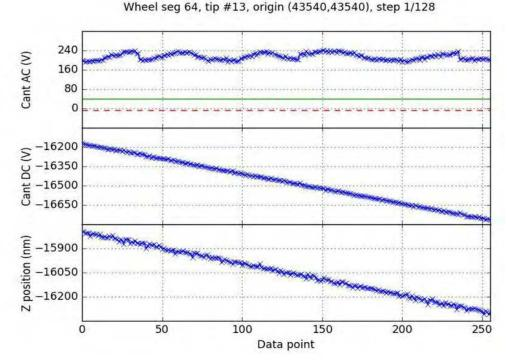
Figure 4: Raw (uncalibrated) control data for a line scan with tip 13 and a wrongly calculated set-point. Note that both the Z position and cantilever DC signals have minimum possible values of -16384, and hence this shows that the piezo was fully extended, resulting in maximum deflection of the cantilever.
