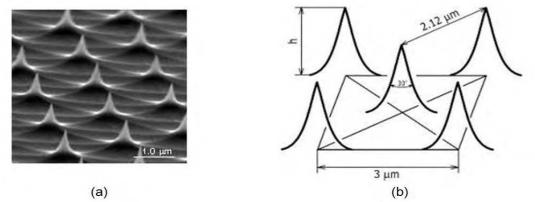
Figure 19: Tip imaging sample mounted at both the flight spare and the flight model. (a) SEM image and (b) schematic illustration showing the dimensions of the sharp tips used for imaging of the AFM tip.
