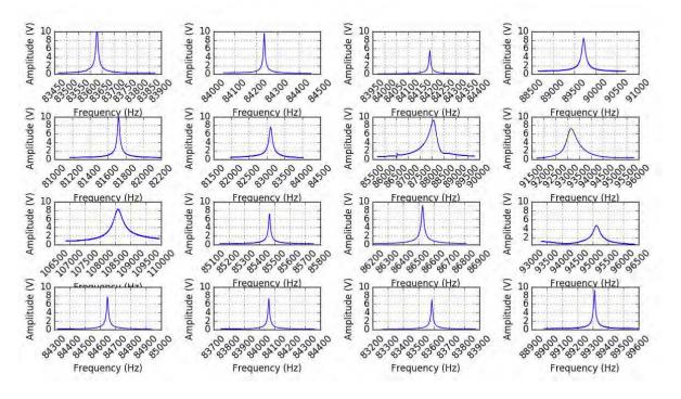
2016-08-21 10:16:00 : Frequency survey of all cantilevers using default parameters
