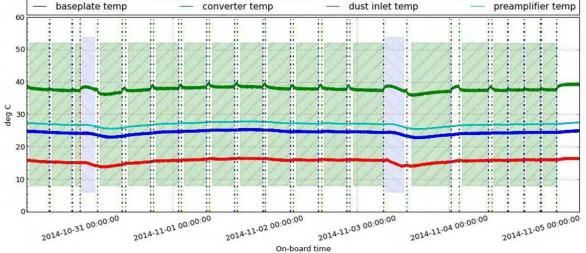
Figure 8: Temperature of the four sensors during STP 26 with most of the time used for scanning (green blocks). At the beginning of the first OCM (blue block) a scan gets aborted due to little time left and MIDAS going to a safe state during the OCM. After both OCM a small increase due to the approach can be observed and after each scan the temperature increases also for approximately 1 °C.
