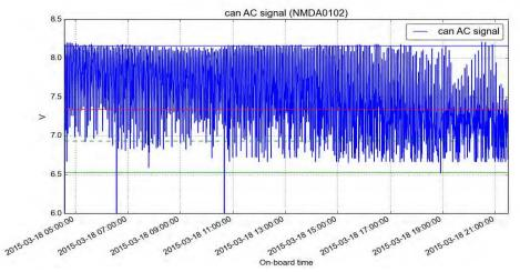
It looks as though the amplitude is often going through resonance. Either the resonance frequency is drifting, or the driving frequency is not stable... Possible ways to improve:
