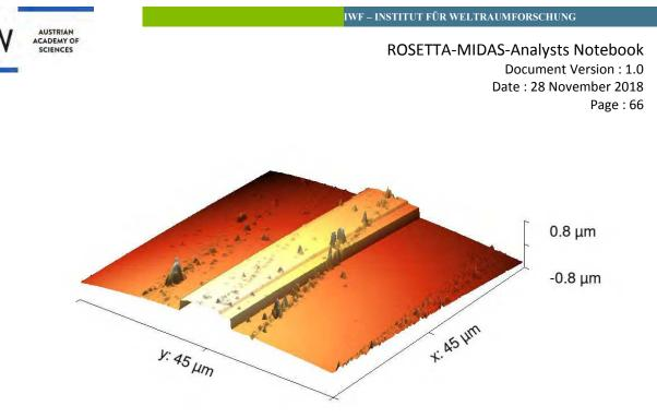
Figure 2. 3D image of STP004-6 showing odd height feature at centre of target and contamination features.
