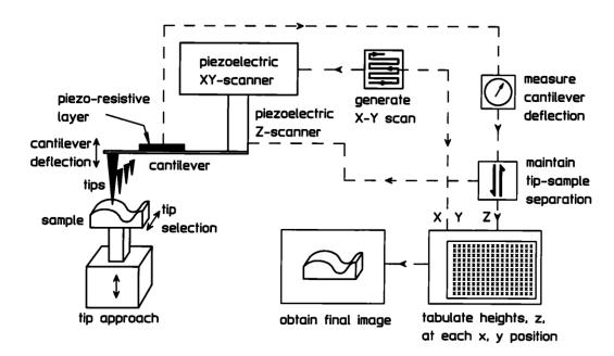
Fig. 2.1 – MIDAS Working Principle
