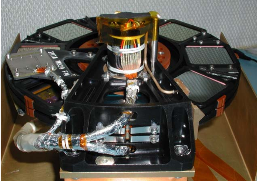
Figure 16. Filter Wheel Mechanism. Two V-shaped flat springs lock the filters by the Vespel cams. Reed switches are activated by encoder magnets to identify the filter in front of the CCD.
