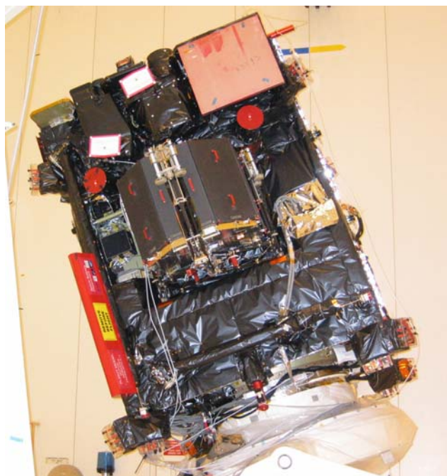
Figure 1. The two OSIRIS cameras units (top left, with white radiators) with VIRTIS and the Philae lander mounted on the -x panel of Rosetta.
