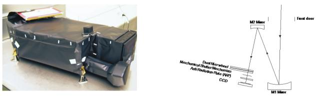
Figure 2: (Left) The OSIRIS WAC flight unit in the lab. (Right) The WAC optical path
