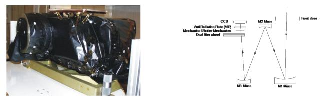
Figure 1: (Left) The OSIRIS NAC flight unit in the lab. (Right) The NAC optical path
