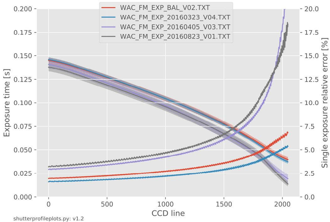
**Figure 5 Average exposure time (left axis) and relative error of the average exposure time for a single shutter activation (right axis) per CCD line as derived from the datasets in Table 3 in the ballistic mode in 4 different configurations. See Table 3 for a definition of the sequences.**
