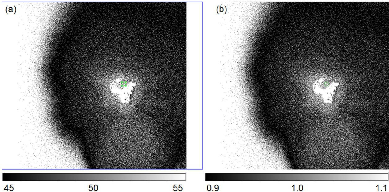
**Figure 6 Ratio of single exposed and 50 exposure stacked images in level 1 (left, a) and level 2 (right, b). Values that are in the level 1 image of the single exposure below the BIAS value + 50 DN are masked, as well as values in the non-linear regime (DN > 45000). The region of interest is shown in green.**
