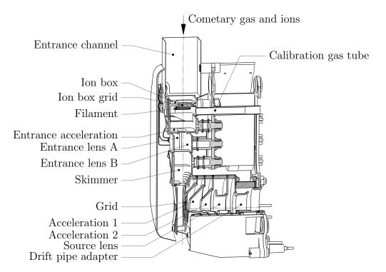
Figure 2.3: Sectional view of the Orthogonal Source.
