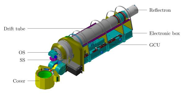
Figure 2.1: 3D drawing of RTOF.
