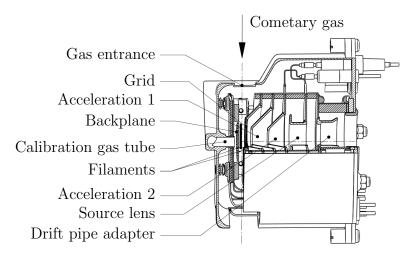
Figure 2.2: Sectional view of the Storage Source.
