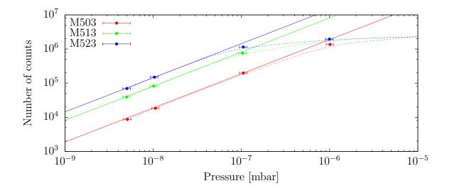
Figure 4.5: Saturation effect for relatively high pressure measurements. A decrease of the  $CO_2$  signal starts to be visible for peaks with a number of counts of  $10^6$ , corresponding to a gas inlet pressure of  $10^{-6}$  mbar for mode 503 but already  $10^{-7}$  mbar for mode 523.
