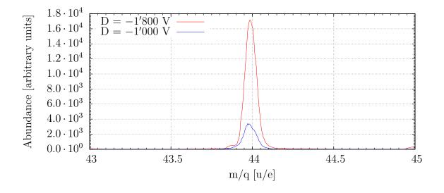
Figure 3.2: Comparison between the RTOF FM settings with D = -1'800 V and with D = -1'000 V, for the OS in mode 513 and a CO<sub>2</sub> gas inlet of  $1.0 \cdot 10^{-7}$  mbar. The red curve for D = -1'800 V corresponds to the red curve from figure 3.1.
