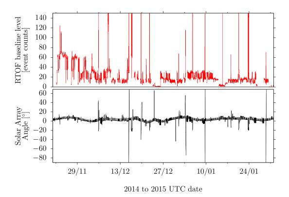
Figure 5.2: Top: intensity of the baseline level for the OS. Bottom: solar array angle. The calculation process is the same as in figure 5.1.
