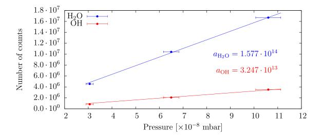
Figure 4.3: Correlation between pressure and number of ions for the parent (H<sub>2</sub>O) and a fragment (OH). A linear interpolation gives a slope of  $1.577 \cdot 10^{14}$  counts/mbar for H<sub>2</sub>O and  $3.247 \cdot 10^{13}$  counts/mbar for OH, leading to the ratio OH/H<sub>2</sub>O = 20.59 %.
