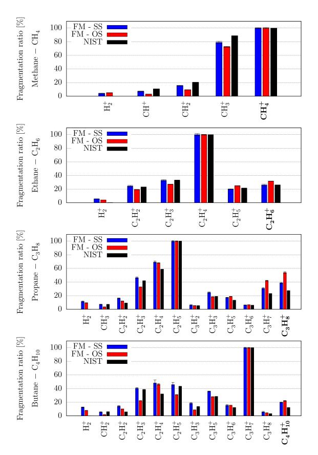
Figure 4.14: Fragmentation ratios - alkanes. Ratios below 5% are not shown, and the labels on the x-axis represent the molecule contributing the most at a given mass.
