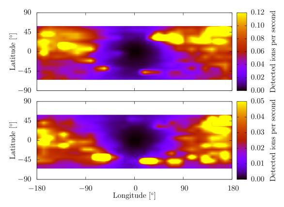
Figure 5.6: RTOF SS  $H_2O$  (upper panel) and  $CO_2$  (lower panel) maps of 67P/Churyumov-Gerasimenko's coma, integrated over the period 01/10/2014 - 01/05/2015. Intensities have been scaled to a distance from the nucleus of 10 km.
