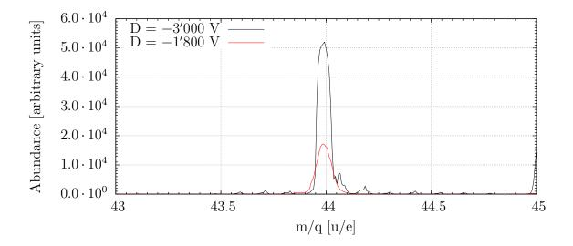
Figure 3.1: Comparison between the initial RTOF FM settings with D = -3'000 V and lowered optimized settings with D = -1'800 V, for the OS in mode 513 and a  $CO_2$  gas inlet of  $1.0 \cdot 10^{-7}$  mbar.
