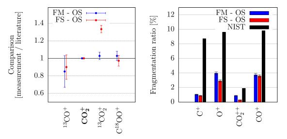
Figure 4.6: Isotopologic and fragmentation ratios for  $CO_2$ . On the left side, the points correspond to the isotopologic ratios measured with RTOF divided by the ones from literature (NIST). On the right side, fragmentation ratios are given relative to  $CO_2^+$ . When not specified,  $C = {}^{12}C$  and  $O = {}^{16}O$ .
