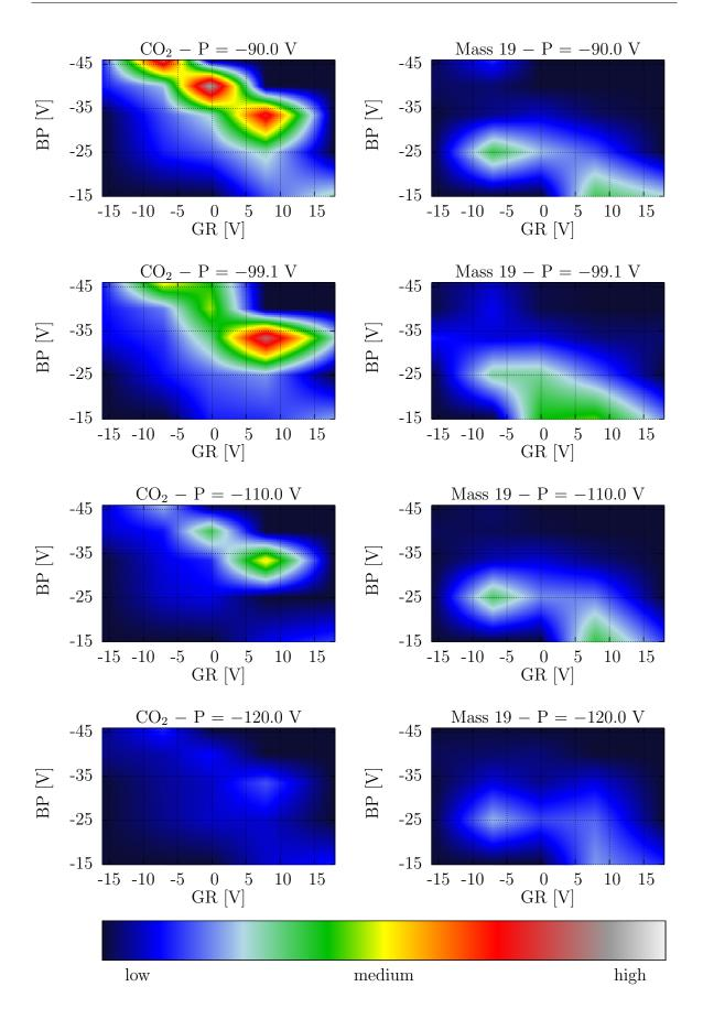
Figure 3.8: Intensity of the  $CO_2$  peak (left) and of the peak at mass 19 (right) with respect to the BP and GR voltages.
