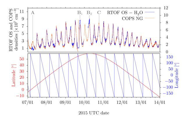
Figure 5.4: Diurnal variations measured by RTOF and COPS in the second week of 2015. Top: RTOF FS densities acquired with the OS for  $H_2O$  (blue) and COPS nude gauge density (orange). Bottom: latitude and longitude of the nadir view of the spacecraft.
