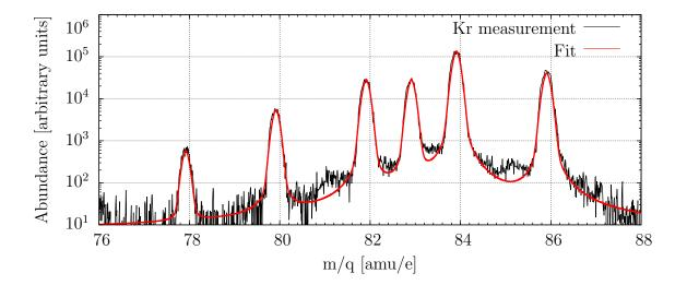
Figure 2.8: Zoom on the krypton isotopes region of a spectrum acquired on ground with the SS with a krypton gas inlet of  $1.0 \cdot 10^{-7}$  mbar. The overlap of the peaks influences the area under the neighboring peaks on the percent level, and therefore fitted together as a sum of pseudo-Voigt profiles.
