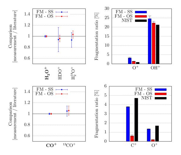
Figure 4.12: Isotopologic and fragmentation ratios for  $H_2O$  and CO. On the left side, the points correspond to the isotopologic ratios measured with RTOF divided by the ones from literature (NIST). On the right side, fragmentation ratios are given relative to  $H_2O^+$  for  $H_2O$ , and  $CO^+$  for CO. When not specified,  $C = {}^{12}C$  and  $O = {}^{16}O$ .
