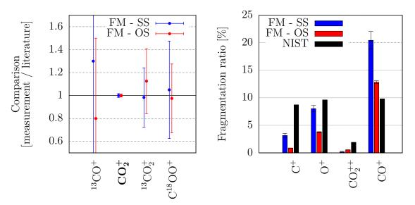
Figure 4.13: Isotopologic and fragmentation ratios for  $CO_2$ . On the left side, the points correspond to the isotopologic ratios measured with RTOF divided by the ones from literature (NIST). On the right side, fragmentation ratios are given relative to  $CO_2^+$ . When not specified,  $C = {}^{12}C$  and  $O = {}^{16}O$ .
