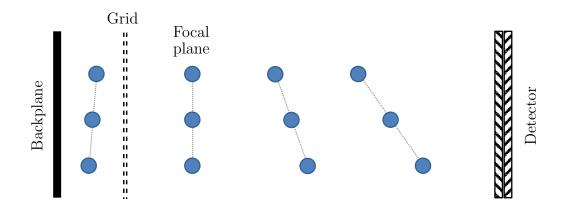
Figure 1.9: The spatial distribution of the ion source causes a spread in travel velocity and a loss in mass resolution.
