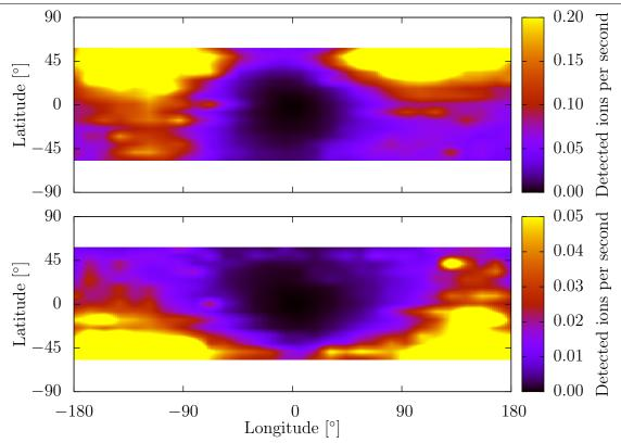
Figure 5.5: RTOF OS  $H_2O$  (upper panel) and  $CO_2$  (lower panel) maps of 67P/Churyumov-Gerasimenko's coma, integrated over the period 01/10/2014 - 01/05/2015. Intensities have been scaled to a distance from the nucleus of 10 km.
