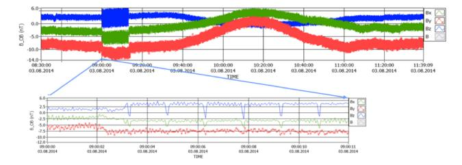
Figure 3.17: Disturbance by thruster activation during OCMs. Besides DC-jumps of  $\sim$ 2 nT additional AC spikes of  $\sim$  6 nT spikes, at  $\sim$  625 mHz, and  $\sim$  200 ms width appear. An automatic cleaning of these structures is hardly possible, but the data in these intervals will be flagged as bad data in the final datasets.
