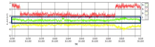
Figure 3.19: Impact of the reaction wheels in the time series. On the upper panel a nice plasma wave structure might be hypothesized (same as Fig 3.16, L3 data). However, a view to the reaction wheel impact eliminated LEVEL H (L4) data in the lower panel clearly depicts, that there are no plasma waves present but only higher frequent disturbances (data shifted due to enhanced visibility).
