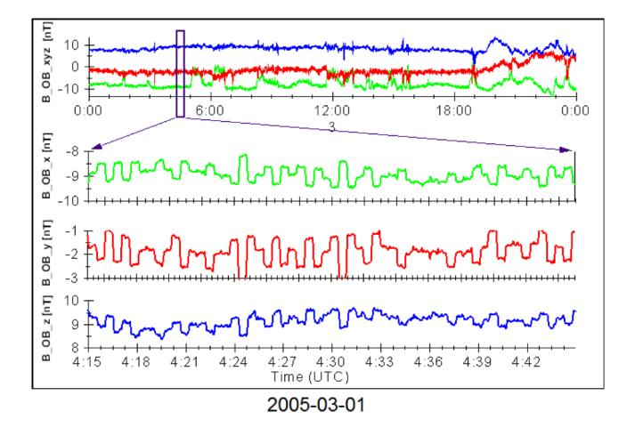
Figure 3.14: Influence of PHILAE heater currents. During the first Earth Fly by heaters on the Lander were activated with 1 min period. The heater current are causing magnetic field disturbances in the order of 1 nT. These disturbances have been accordingly flagged in the dataset. Unfortunately, they cannot be removed.
