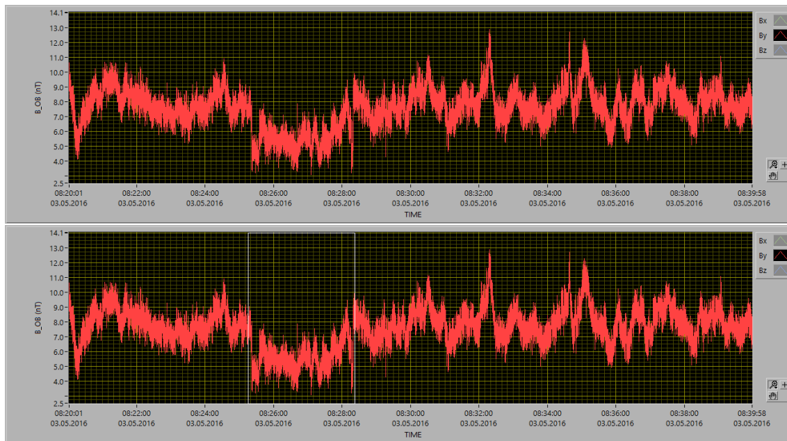
Figure 2: Examples of a WOL disturbance recorded on 03.05.2016 during the EXT2 phase with the OB sensor. Top: The x-axis shows time, the y-axis shows the y-component of the magnetic field. Bottom: The white box marks the duration of the WOL disturbance.
