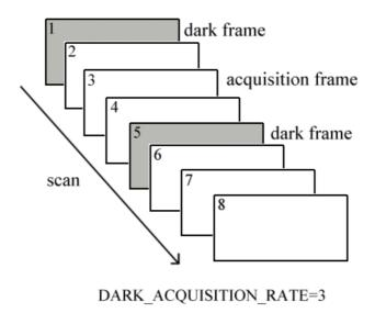
Figure 4-2: Structure of dark frames acquisition.
