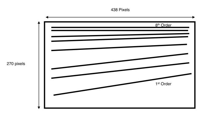
Figure 2-3: Spectral orders distributed over the IR FPA area. Only 15% of the matrix contains scientific data.
