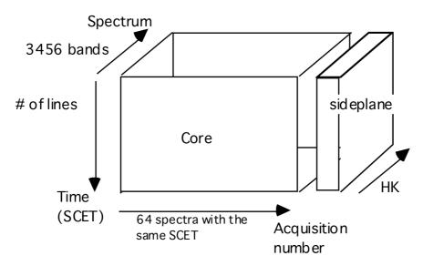
Figure 4-3: VIRTIS H data cube in 64-spectra mode. In this case, each frame contains the 64 spectra transferred together. The # of bands is equal to 3456.
