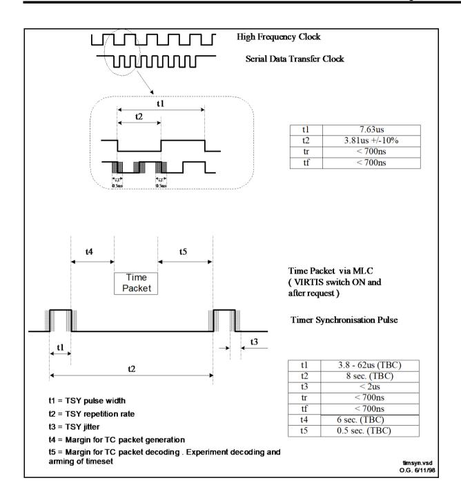
Figure 2.10 DMS timing & synchronisation signal (OTS) timing
