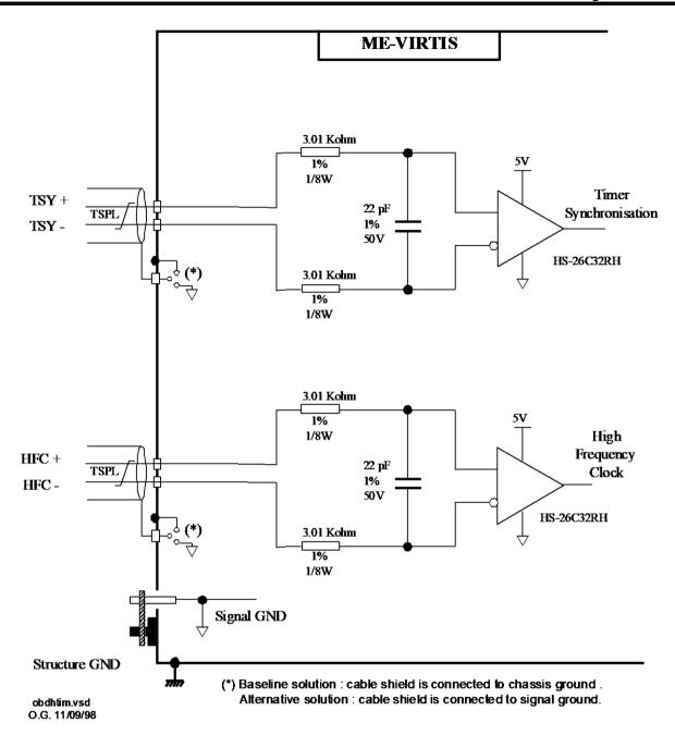
Figure 2.9 DMS timing & synchronisation signal (OTS) interface circuit
