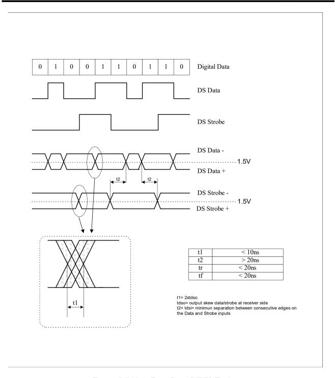
Figure 2.7 High Rate Data (HRD) Timing
