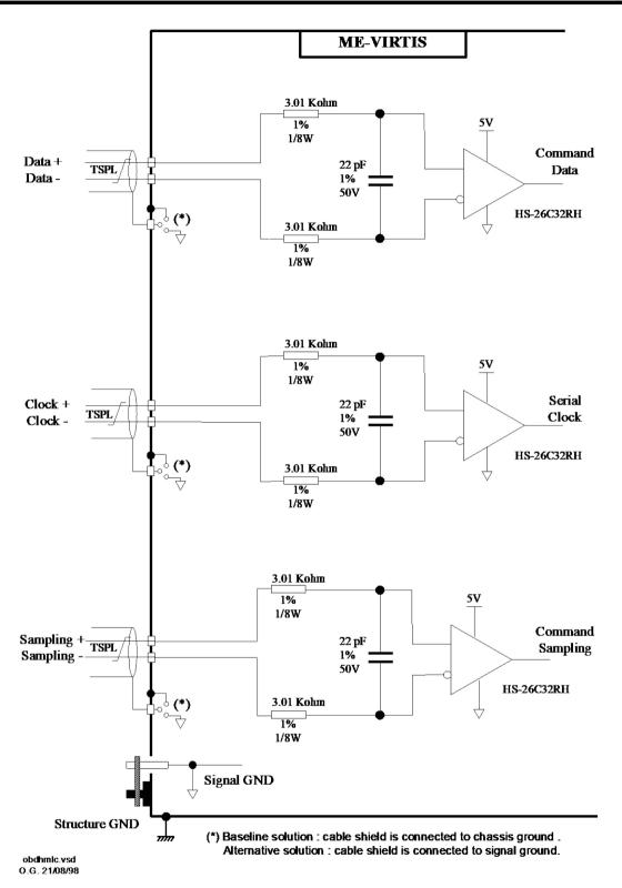
Figure 2.2 MLC (Memory Load Command) interface circuit
