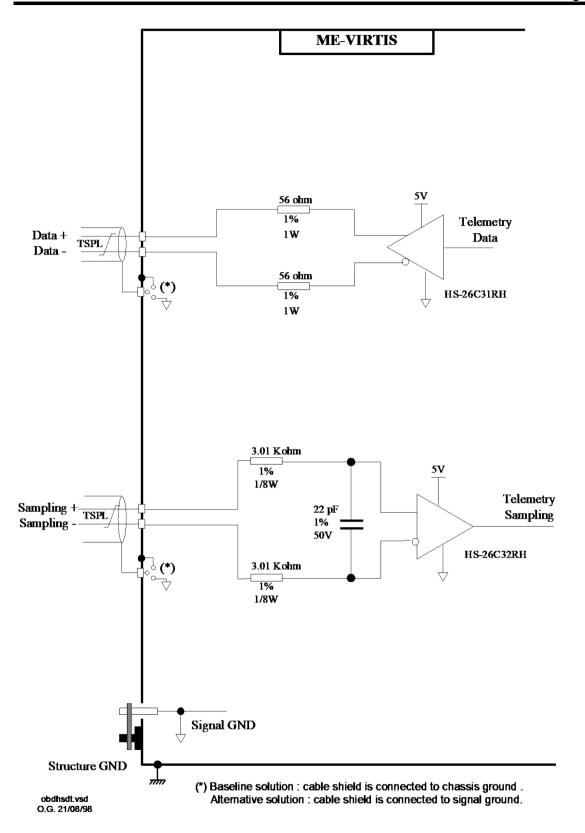
Figure 2.4 16Bit Serial Digital Telemetry (SDT) interface circuit
