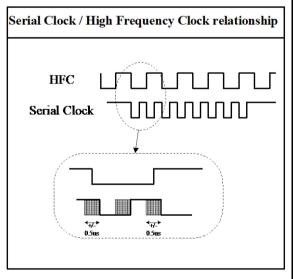
Figure 2.5 16Bit Serial Digital Telemetry (SDT) timing
