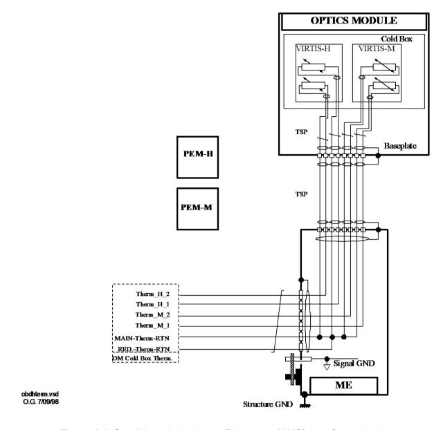
Figure 2.8 Conditioned Analogue Telemetry (ANC) interface circuit
