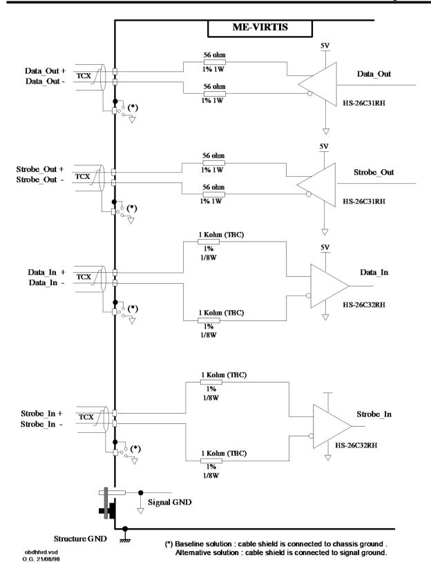
Figure 2.6 High Rate Data (HRD) link interface circuit
