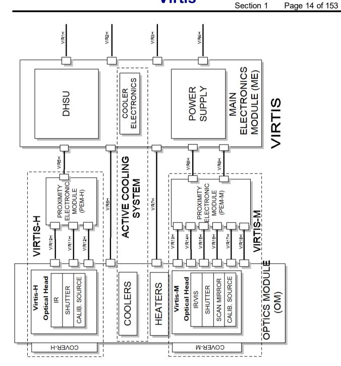
Figure 1.1 VIRTIS Functional Block Diagram
