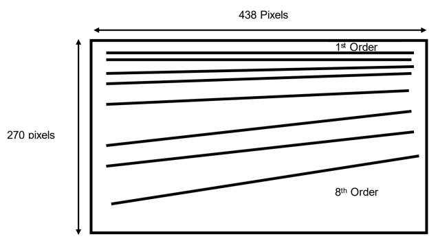
Figure 3.2 Spectral orders distributed over the IR FPA area. Only 15% of the matrix contains scientific data.
