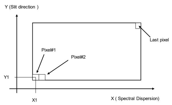
Figure 3.4 Data Organisation on the CCD and IR detectors of VIRTIS-M
