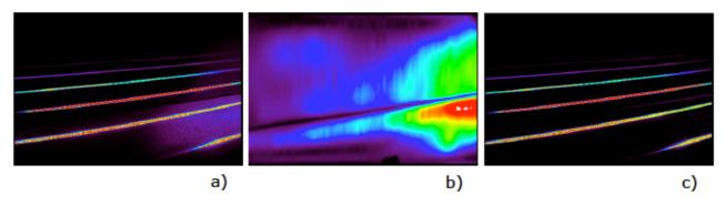
Figure 12: a) Backup raw image (2D) - b) map of the stray light - c) Backup raw image corrected from the stray light effect
