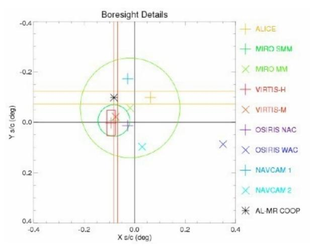
Figure 6: Details of Rosetta instruments' FOV in the spacecraft X/Y frame. Zs/c points into the page, +Xs/c points to the right, and +Ys/c points down (figure from AD3)
