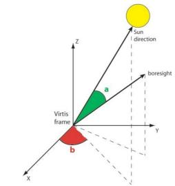
Figure 4: Sun direction in the instrument frame
