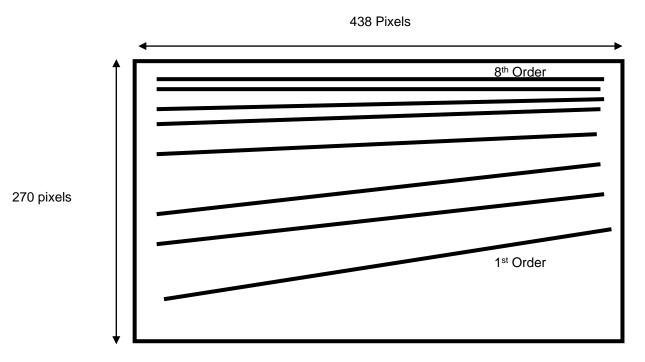
Figure 2.3 Spectral orders distributed over the IR FPA area. Only 15% of the matrix contains scientific
