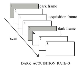
Fig. 4.2 – Structure of dark frames acquisition
