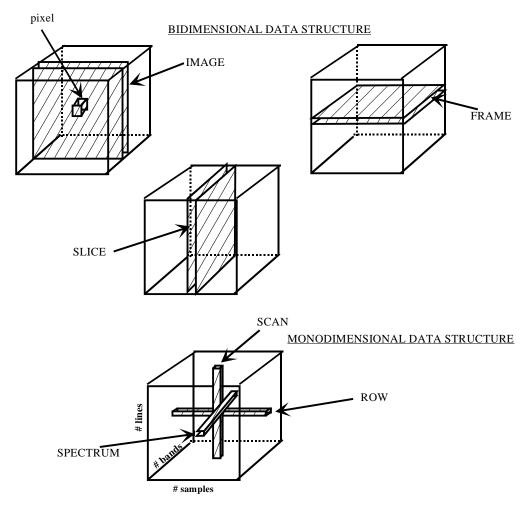
Fig. 4.1 - Structure of the qube data
