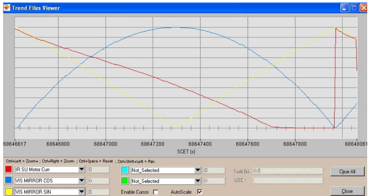
Figure 10. H/K Mirror COS (yellow), SIN (Blue) and motor current (red). It can be noticed that at about time (on the X axis) 68647700 the red curve saturates. Boresight location is at about time 68647300.
