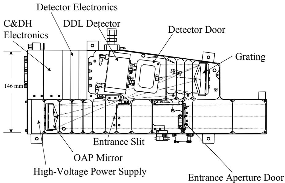
Figure 2-1: The opto-mechanical layout of *Alice*.
