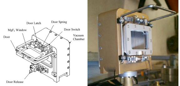
Figure 3.1-2. (Left) Schematic of the Alice DDL detector vacuum housing; (Right) Photograph of the PFM DDL detector vacuum housing.
