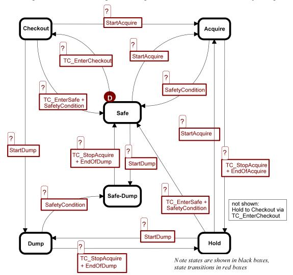
Refer to Figure 2.3-2 for a state diagram showing the transitions between the *Alice* operating states.
