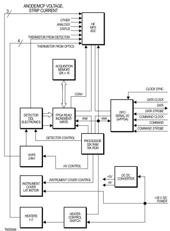
Figure 3.1-3. The Alice electrical block diagram.
