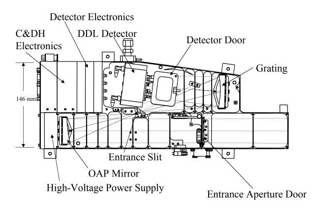
Figure 1.3-1. The opto-mechanical layout of Alice.
