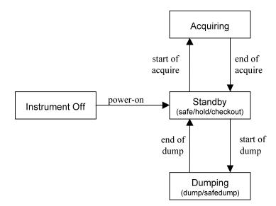
Figure 4.1-1. The Alice top-level mode transitions.
