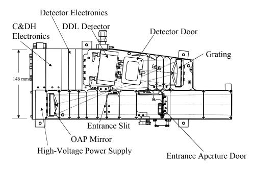
Figure 2-1: The opto-mechanical layout of Alice.
