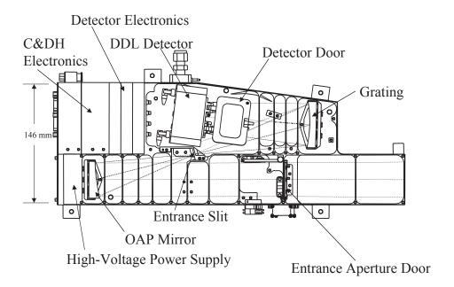
Figure 2-1: The opto-mechanical layout of Alice.
