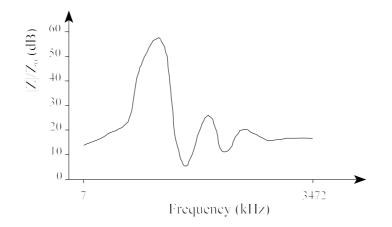
Figure 1. Example of mutual impedance probe response versus frequency (normalized square modulus).
