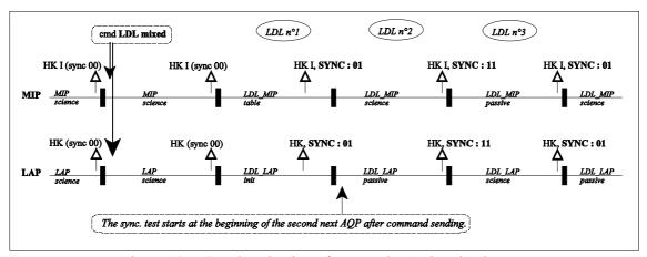
Figure 13-a. Synchronization of MIP and LAP in mixed LDL.
