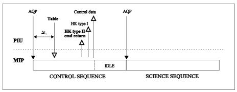
Figure 8. Command return with HK type II when the configuration table is received during the switching on procedure.
