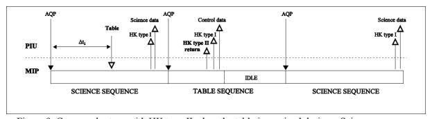
Figure 9. Command return with HK type II when the table is received during a Science sequence.
