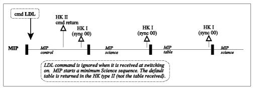
Figure 15. LDL command not received in a Science sequence.
