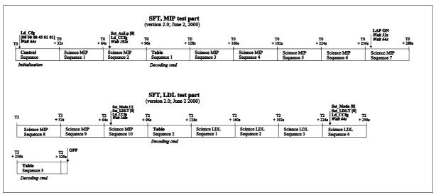
Figure A3.3.1. SFT: Time diagrams for the MIP and LDL (type 0 only) parts.
