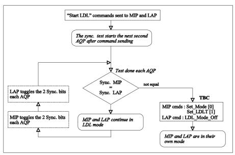
Figure 12. MIP and LAP synchronization.
