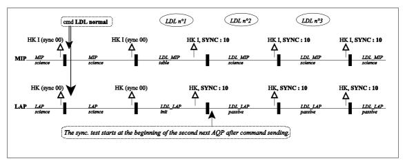
Figure 13-b. Synchronization of MIP and LAP in normal LDL.
