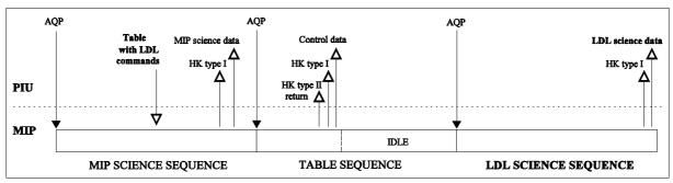
Figure 11. LDL mode command received during a MIP science sequence.
