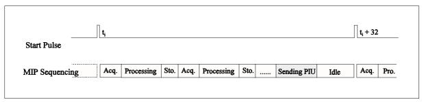
Figure 4. Details of a MIP Science sequence. The three main tasks, signal acquisition from the sensor, processing and data storage into RAM, are successively run. The data sending to PIU is done before the reception of the next start pulse (HK data first, then science data).
