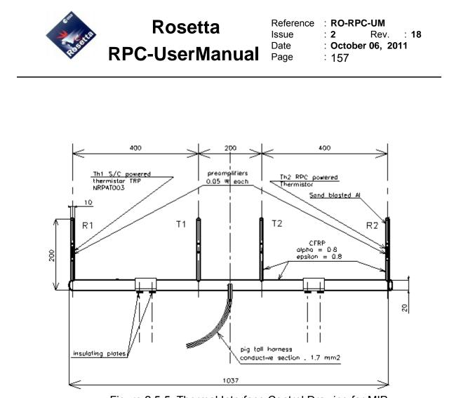
Figure 2.5-5: Thermal Interface Control Drawing for MIP
