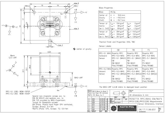
Figure 2.1-9: MAG Sensor Dimensions
