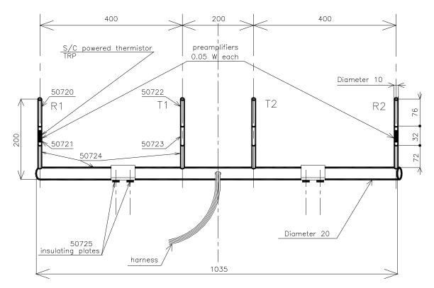
Figure 2.5-13: MIP Sensor Thermal Sketch
