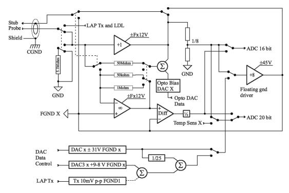
Figure 1.2-4 LAP diagram for the input stage of one of the two probes.
