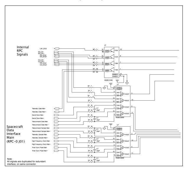
Figure 2.2-2: SDBL Interface Circuits
