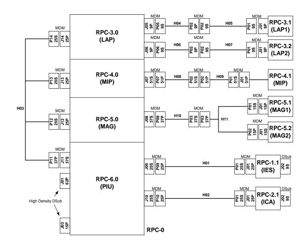
Figure 2.1-1: RPC Experiment Layout and Harness Diagram
