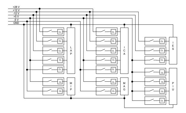
Figure 2.2-1: RPC Power Distribution Block Diagram
