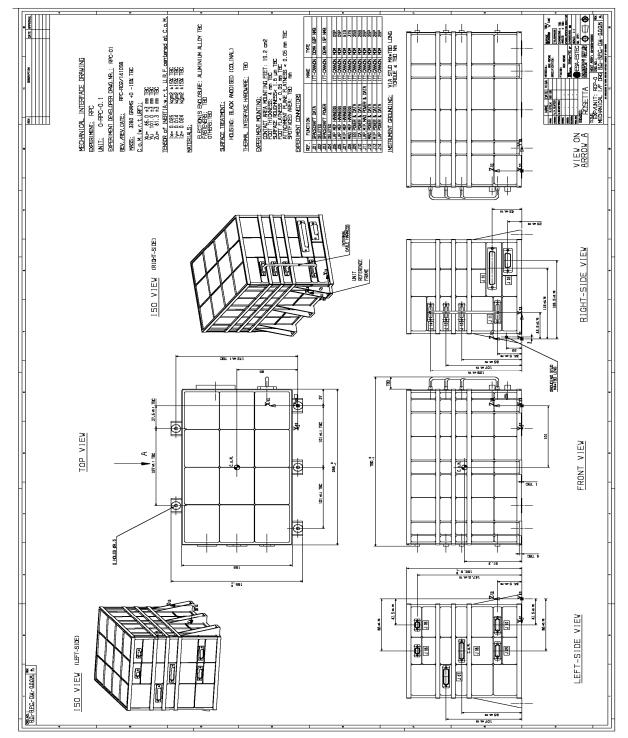
Figure 2.1-2: RPC-0 Mechanical Interface Drawing
