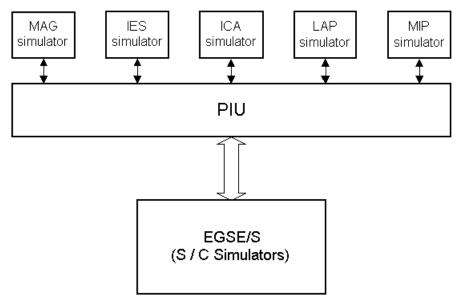
Figure 3.5-2: Autonomous Test of the PIU
