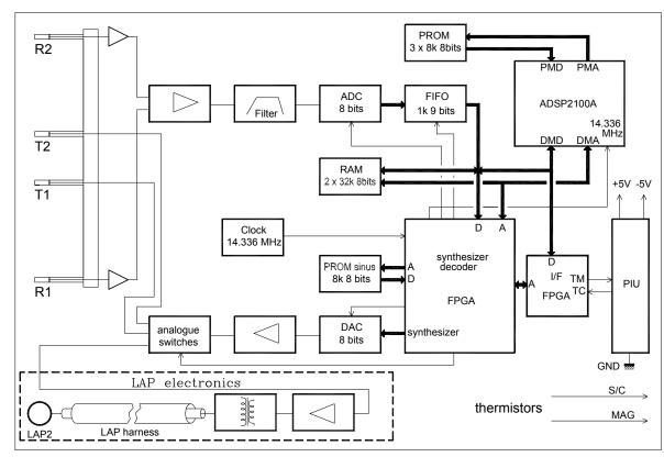
Figure 1.2-10: Mutual Impedance Probe (MIP) Block Diagram
