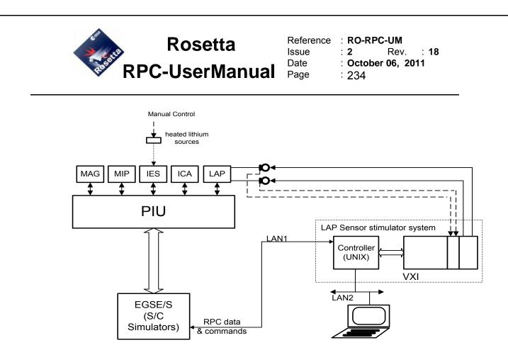
Figure 3.5-3: System Level Test of the Rosetta Plasma Package
