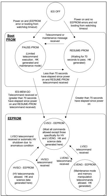
Figure 4.1-2: IES Mode Transition Diagram.
