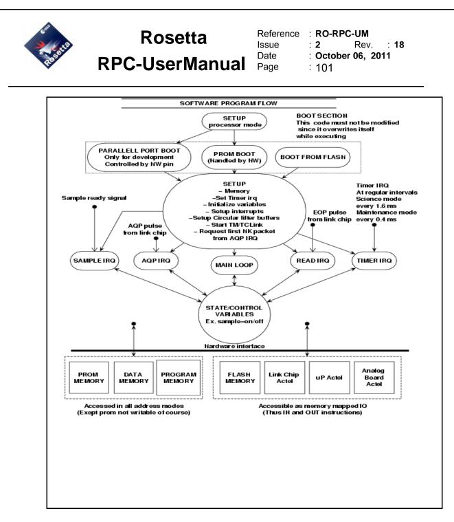
Figure 2.3-6: LAP Software Structure
