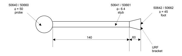
Figure 2.5-12: LAP1 and LAP2 Thermal Sketch
