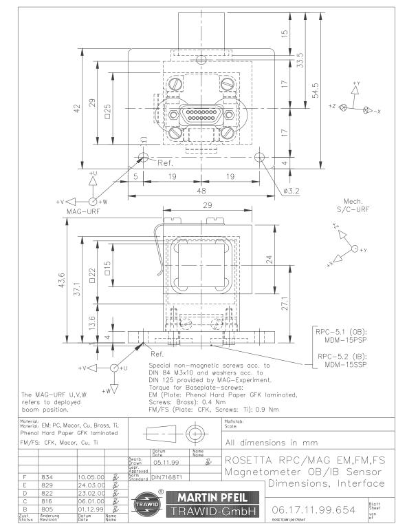
Figure 2.1-12: MAG Sensor Dimensions, Interface
