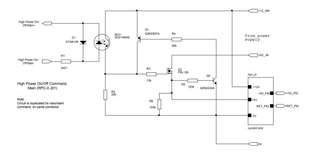
Figure 2.2-3: High Power Command Interface Circuit
