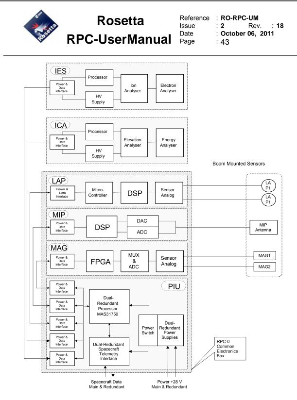
Figure 1.2-1: RPC Overall Block Diagram
