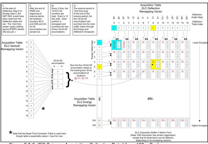
Figure 2.3-3: IES Science Acquisition Collection Detail for a 128 s Cycle
