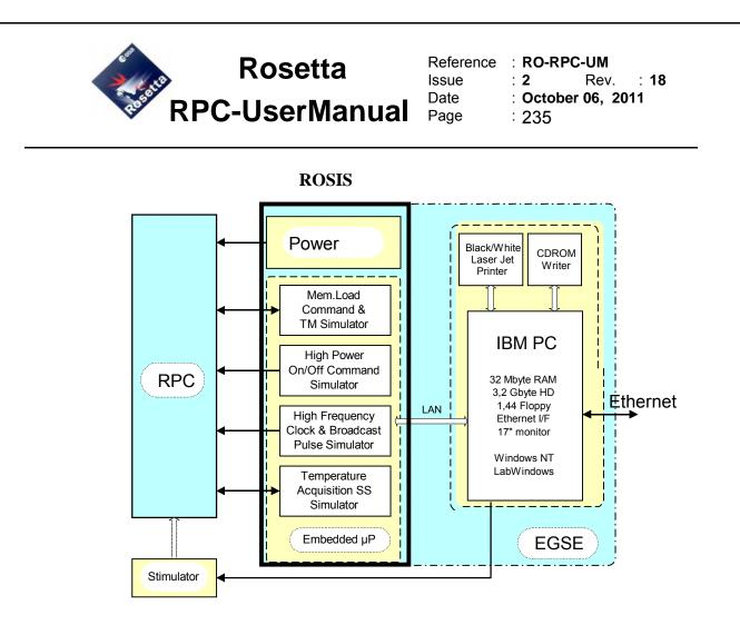
Figure 3.5-5: RPC Experiment Level testing with the ICSTM EGSE
