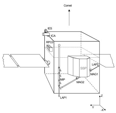
Figure 1.2-2: RPC Sensors Layout (stowed)
