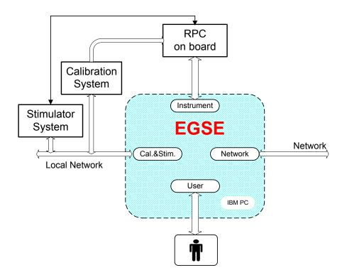
Figure 3.5-4: Logical Interfaces of the ICSTM EGSE
