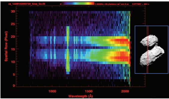
*Figure 7.* Example of an Alice histogram (left) of 67P and a NavCam context image [12] with an overlaid Alice FOV (right) acquired on 08/18/2014 (2014 DOY230). The context image can help identification of scene characteristics to correlate histogram features.
