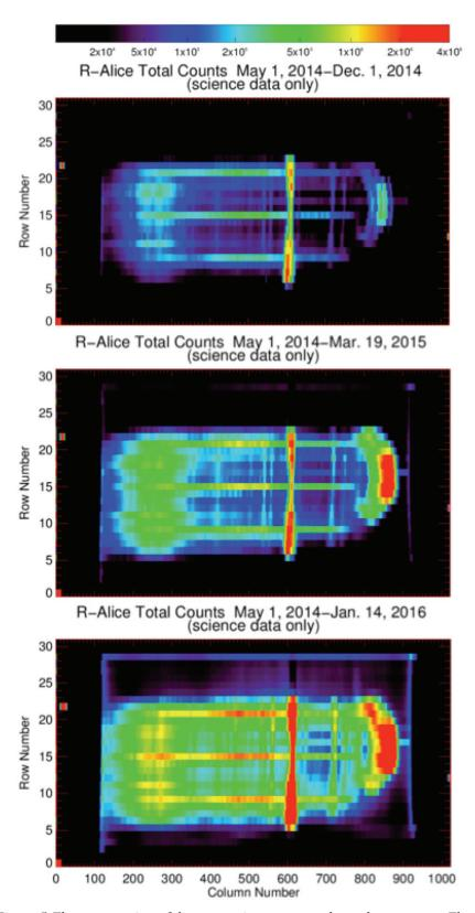
Figure 5. The progression of detector science counts through encounter. The concentration of counts near column 600 (1215 A) is the Ly- $\alpha$  line and the region around column  $\sim\!850$  ( $\sim\!1025$  Å) corresponds to the chameleon artifact region. The high concentration of counts in rows 9, 15, and 21 are due to stellar calibrations. Wavelength decreases to the right, i.e., to higher row number.
