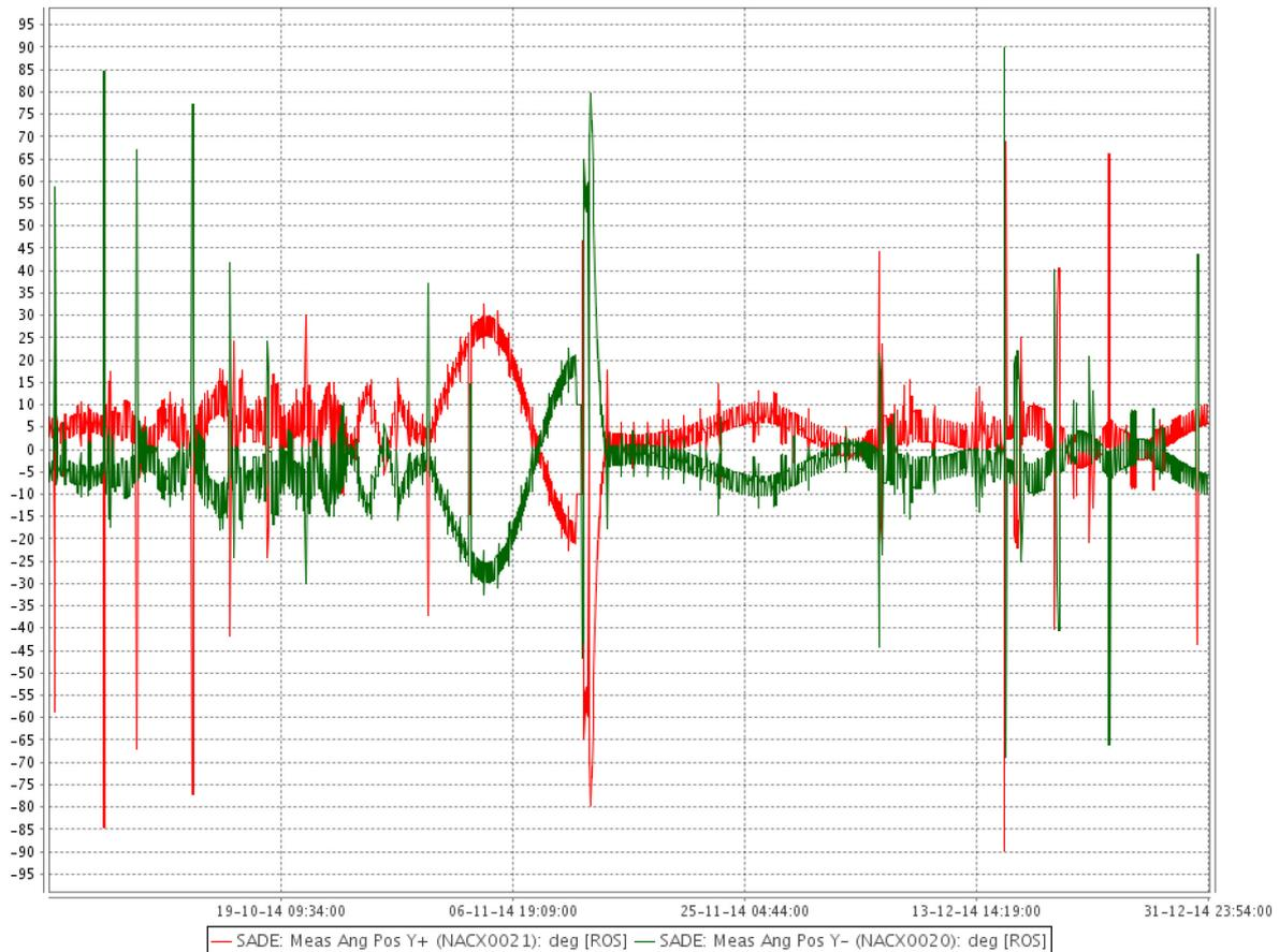
**Figure 35 : Measured angular position of the solar panels – Q4 2014**
