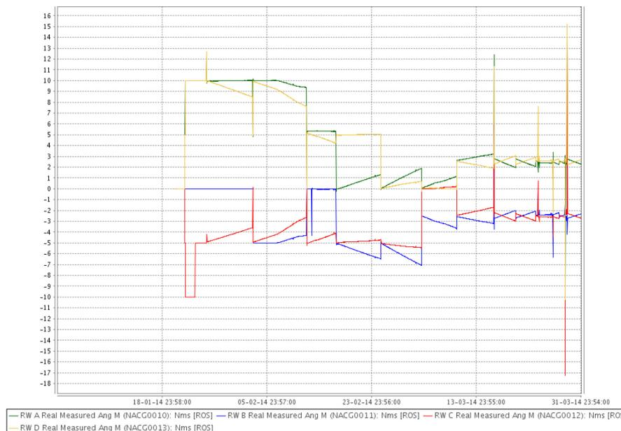
**Figure 19 : Reaction wheel angular momentum**
