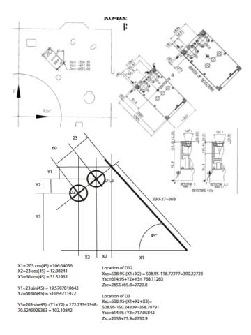
Figure 3. Combination of geometry info to calculate SREM head locations (centre) in sc coordinates.
