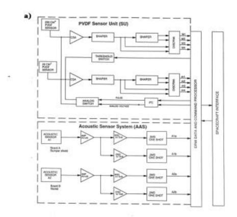
Figure 3. Block diagram of the principal electronic functions of the DFMI.
